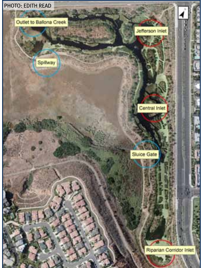
Figure 2. Design Features of the Freshwater Marsh
